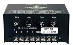
d. From your load (lighting) hook up the white wire (common) to the terminal marked "COM" TO CHASE LIGHTING.
